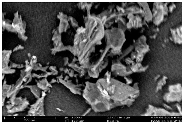
**Figure 3:** Scanning electron micrograph of PAAC before adsorption
