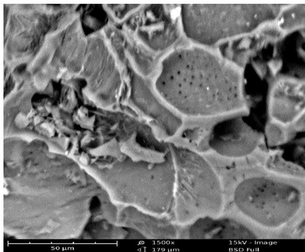
**Figure 4:** Scanning electron micrograph of PAAC after adsorption
