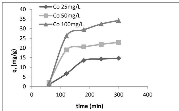
Fig. 2 : Batch adsorption of MY on PAAC derived from *G. aborea* bark at 29°C at various  $C_0$
