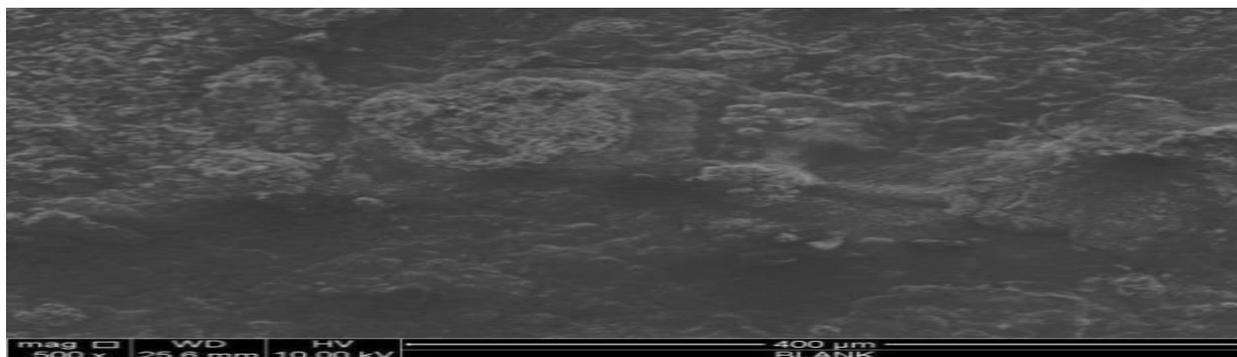
Plate I: SEM of the mild steel treated with 5mol/dm<sup>3</sup> HCl for 5h without inhibitor
