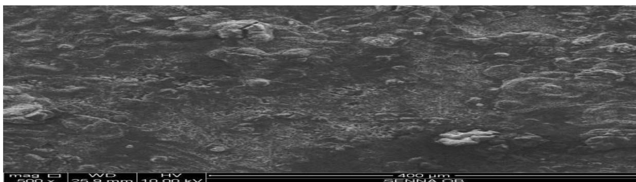
Plate II: SEM of the mild steel treated with 5mol/dm<sup>3</sup> HCl for 5h in the presence of 0.1%w/v of extract of *Senna obtusifolia* inhibitor
