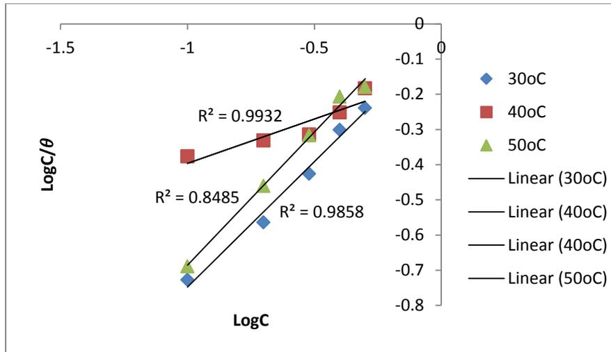
Figure 1: Langmuir isotherm of *Senna obtusifolia* extracts on mild steel in  $5\text{mol}/\text{dm}^3$  HCl at difference temperature
