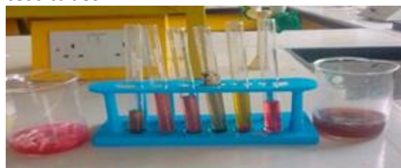
Figure 3: progressive formation of copper nanoparticles after the addition of copper nitrate solution to aqueous extract of Costus afer . Beakers labelled B_R and B_L contain precipitated CuNPs solution and plant extract respectively. Each of the test-tubes labelled 1 to 6 from right contain copper nanoparticles, 2 ml of extract, 2 ml of extract and 0.1 ml of copper solution, 2 ml of copper solution and 2ml of extract, 2 ml of extract and 0.5 ml of copper solution, 2 ml of extract and 1 ml of copper solution
