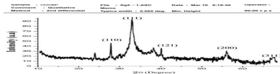
Figure 1b: XRD Diffractograms of Isolated Cellulose of PMBP
