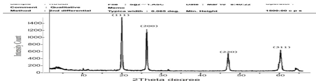
Figure 1b: XRD Diffractograms of Raw Cellulose of PMBP)
